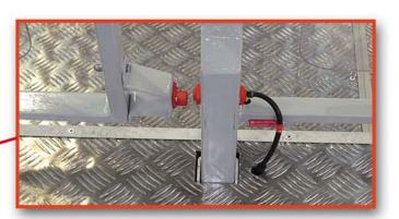
The ride is equipped with entry and exit stairs with safety sensors monitoring access to the ride and stopping the ride in case doors are open.
